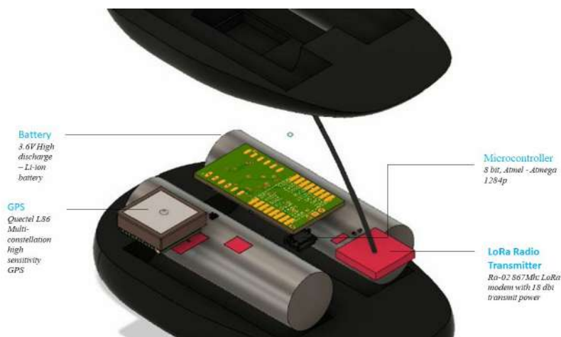
Figure 8. Components of the GPS-LoRa tag.
